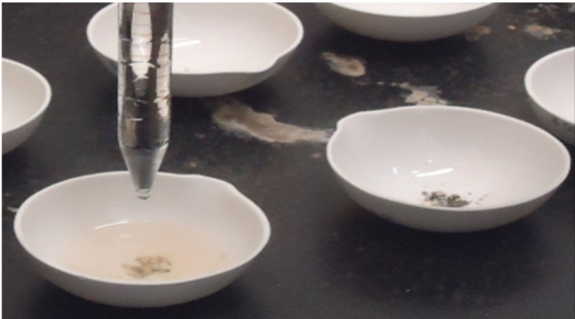
Figure 2 Samples are dissolved with heated 10 ml of HCl 10M, then mixed with HNO 3 0.1M until it reached 100 ml
